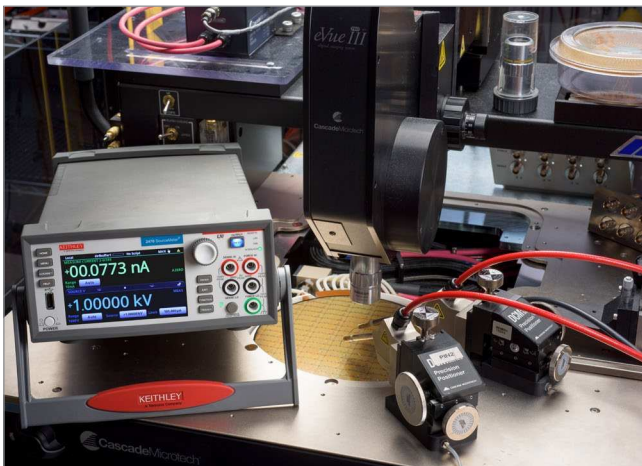
Characterize transistors with multiple SMU instruments on wafer or packaged transistors
